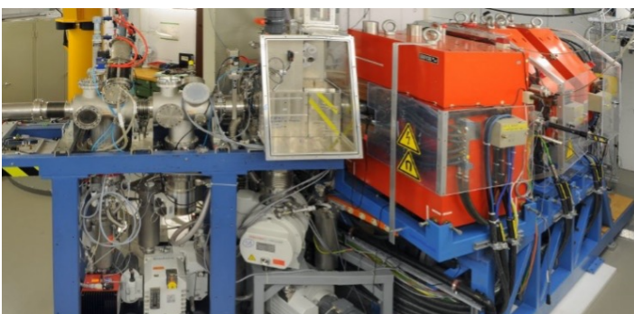
The gas-filled recoil separator used to synthesize rutherfordium-252.
