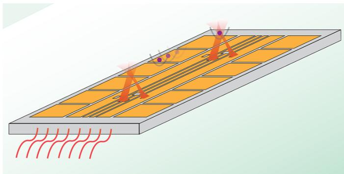
**Figure 1:** Mordini and colleagues present building blocks for a quantum computer whose quantum bits are trapped ions (purple) [6]. Individual ions are transported above surface electrodes (light orange), which are patterned on a dielectric material (light gray) and have integrated photonics underneath. Light enters the system through optical fibers (red) and is sent to two separate zones where it is launched as a pair of crossing beams (dark orange) to manipulate an ion's state.
