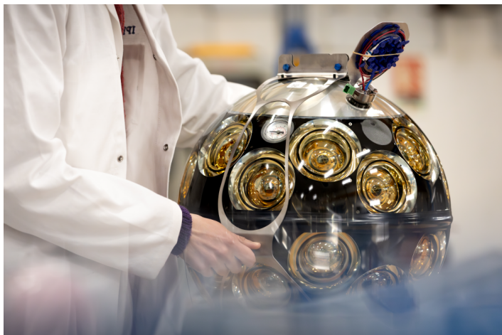
One of the optical-sensor modules being calibrated in the lab. Credit: CNRS/N. Busser
