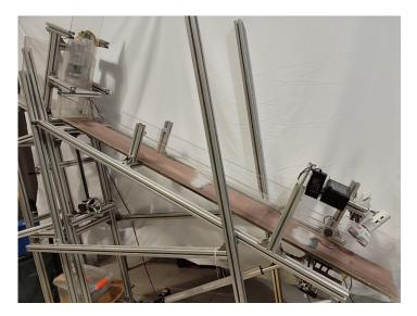
**Sand slide.** The experimental setup consists of a hopper (upper left) that releases grains down an inclined board. The speed of the grain flow is measured by a camera (bottom right). **Credit: Y. Wu/Zhejiang University**
