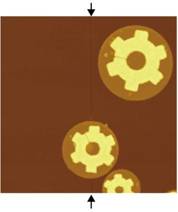
**Sliding gears.** Sliders 2–4  $\mu$ m in diameter made of multilayer graphene are topped with a palladium "gear" structure (yellow) in order to reveal the crystal lattice's orientation and provide a contact point for the sliding arm. The research team measured the influence of edges by dragging the sliders over a crack (vertical line at arrows) in the underlying surface.
