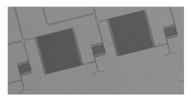
This micrograph image shows a counting device for a single-photon detector. In this new design, both the detector and the signal processing electronics are fabricated from superconducting nanowires.
