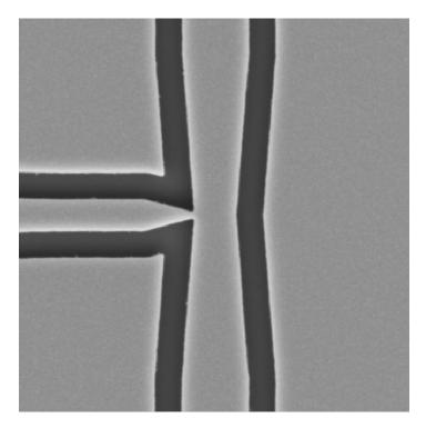
A close-up view of a nanocryotron (nTron) consisting of three superconducting nanowires. The bottom nanowire is the source, the top is the drain, and the thinnest wire on the left is the gate. These devices have now been incorporated in a cryogenically cooled counter for single-photon detectors.
